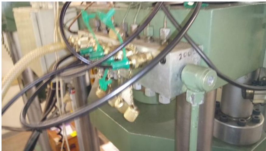
Figure 13 - hydrostatic bearing feed valve (200 kN)
